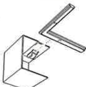
TK 107 Horizontal Elbow Assembly for TKN Track.
