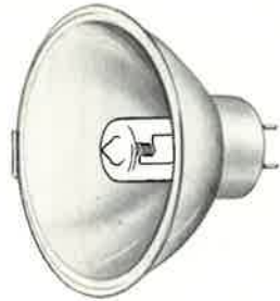
A1/229 8V 50W Tungsten Halogen Lamp The A1/229 has been designed particularly for Super 8 cine projectors. It is a complete optical system comprising a tungsten halogen lamp integral with an aluminised ellipsoidal mirror reflector. Equipment utilising this light source is able to dispense with the conventional condenser optical system, and this results in an appreciable gain in the level of screen illumination. The design permits extremely accurate alignment of the lamp within the projector.
